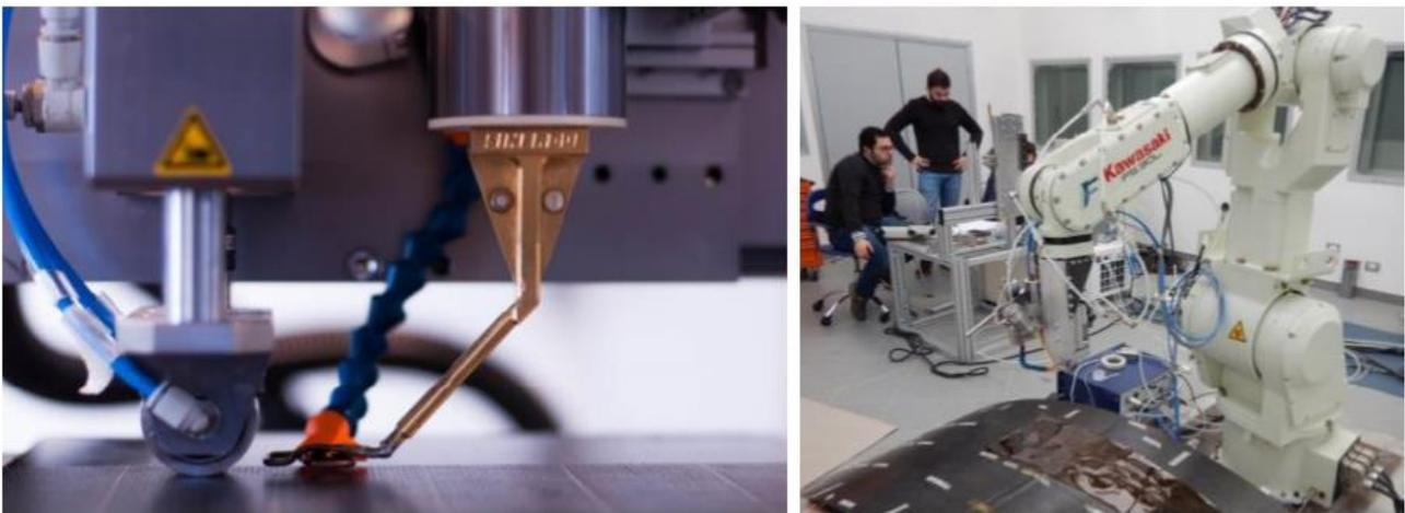
Figure 2 View of the induction welding equipment developed by CETMA
