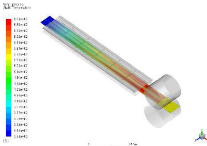
Figure 1 CFD model results - Temperature on prepreg
